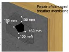
Damage should be repaired thoroughly by removing damaged material and installing a new piece of applicable membrane pushed under the existing membrane and then passing over the existing membrane (see image) with 150mm (6") overlap to sides of hole and 100mm (4") at top/bottom. The membrane should be sealed using CON-EXO, ECHOSEAL or VARASEAL to connect the overlap.
