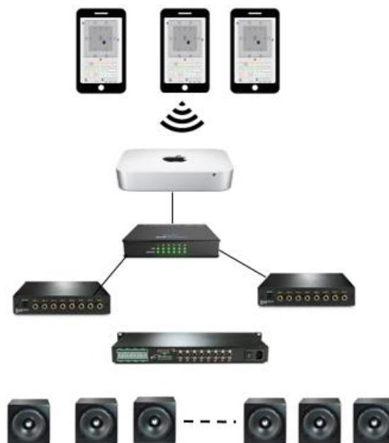
**Fig. 1:** A typical Immergo immersive sound system configuration
