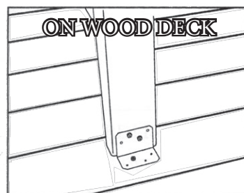
Use Simpson A-23 4 - 1" Screws per post
