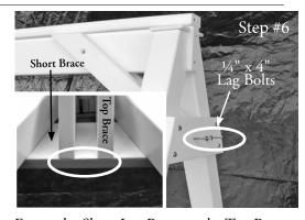
Fasten the Short Leg Brace to the Top Brace using  $\frac{1}{4}$ " x 4" Lag Bolts (and  $\frac{1}{4}$ " Washer). As shown in the inset, ensure that the bottom of the Short Brace is even with the bottom edge of the Top Brace.
