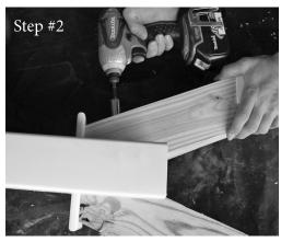
Tighten Nuts using a 3/8" socket and cordless drill.
