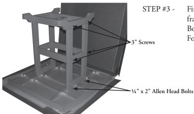
First fasten the second Base to the aluminum frame of the Top using ¼" x 2" Allen Head Bolts. Second fasten the Cross Support and Footrests to the Base using 3" Screws.
