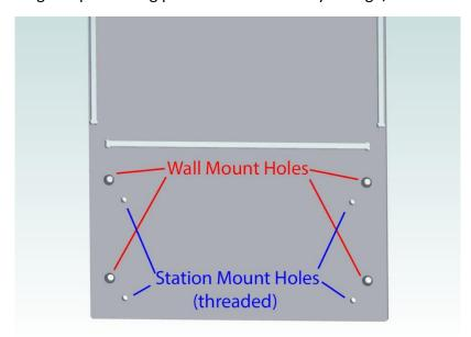
2. Once the sign bracket is mounted securely to your wall, position hygiene station to bracket and align 4 square cut-outs in the back of the station with the 4 threaded Station Mount holes on the sign bracket. Use the 3/8" long button head screws to mount station to wall bracket/sign in the 4 threaded holes.
