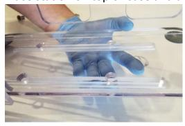
3. Insert 5/16-18 x ¾" screw and finger tighten.
