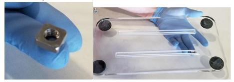
2. Place station on top of base and align square nut hole with station hole.
