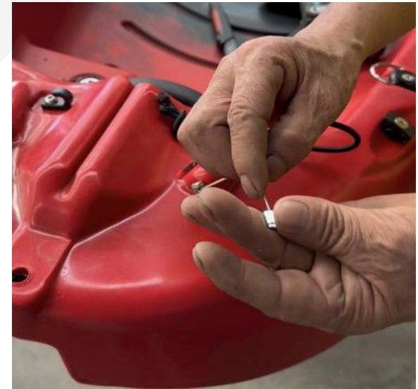
6 Thread the cable through the screws and the safety pin.
