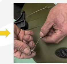
5 Thread the cable through the butterfly screws and fixing bolt.
