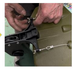
7 Attach the butterfly screws to the stern rudder.
