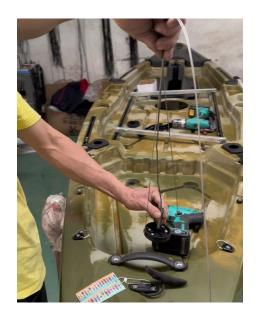
Use the iron wire to pull the controller through the square hole.
