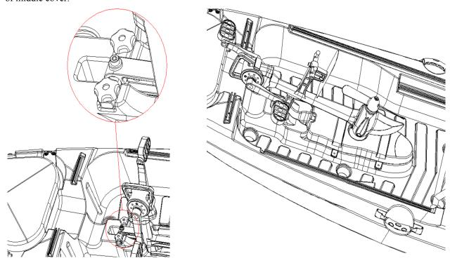
Once in deep enough water, remove the black cover and lower the pedal drive unit down, locking the bolt part (5-c) into place (as illustrated below). Then close the cover to keep kayaking.
