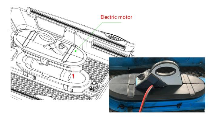
3. Connect the two ribbon ties and connect the power interface.
