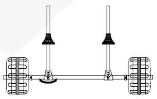
3. Put the tube into the hole on the top. Adjust the distance between the two tubes according to the drain holes on the kayak. Tighten the nut to prevent the tube to move.
