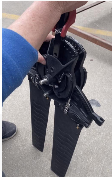
4. Slide the foot pedal down until the holes line up
