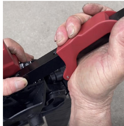
3. Press the red reinforcement button
