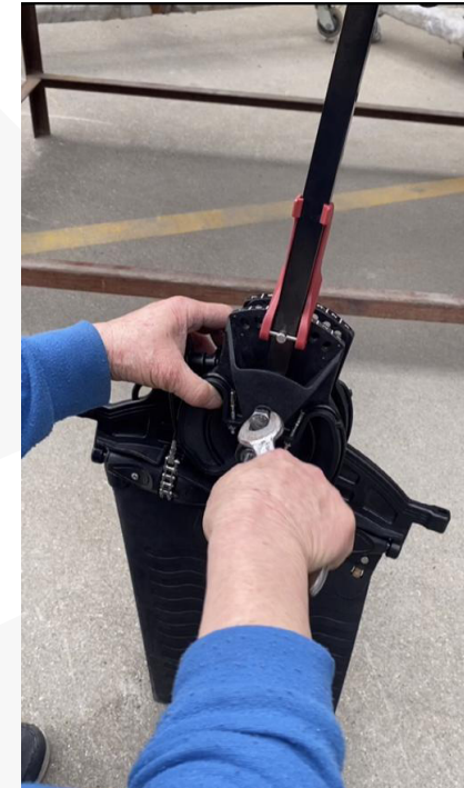
6. Insert bolt and secure by hand or spanner
