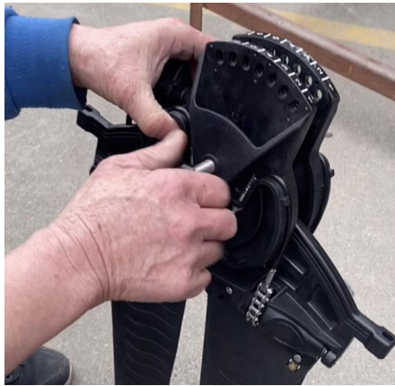
2. Remove the bolt from drive seal
