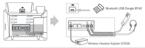
Note: The headset, Bluetooth USB dongle BT40 or wireless headset adapter EHS36 should be purchased separately. The EXT port can also be used to connect the expansion module EXP40. For more information on how to use the EHS36, EXP40 and BT40, refer to Yealink EHS36 User Guide, Yealink EXP40 User Guide and Yealink Bluetooth USB Dongle BT40 User Guide.
