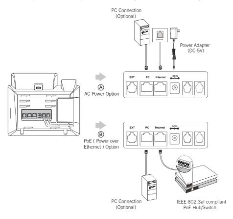
Note: The IP phone should be used with Yealink original power adapter (5V/2A) only. The use of the third-party power adapter may cause the damage to the phone.
