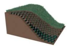
There is a 'correct' and a 'wrong' direction for installing Slope Grid. Slope Grid consists of long strips that are welded together at intervals. The long strips need to be parallel to the hillside.
