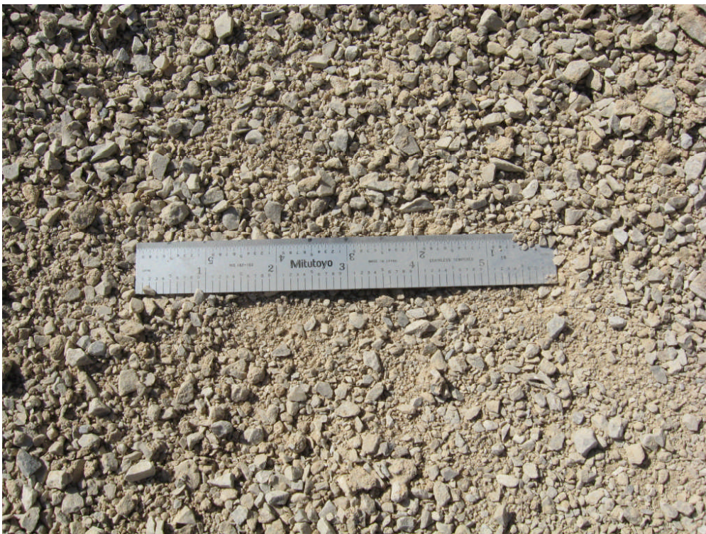
Figure 4-4. Installation damage Type 3 test aggregate.
