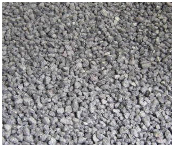
Figure E-2. ISO/EN 10722, laboratory installation damage aggregate.
