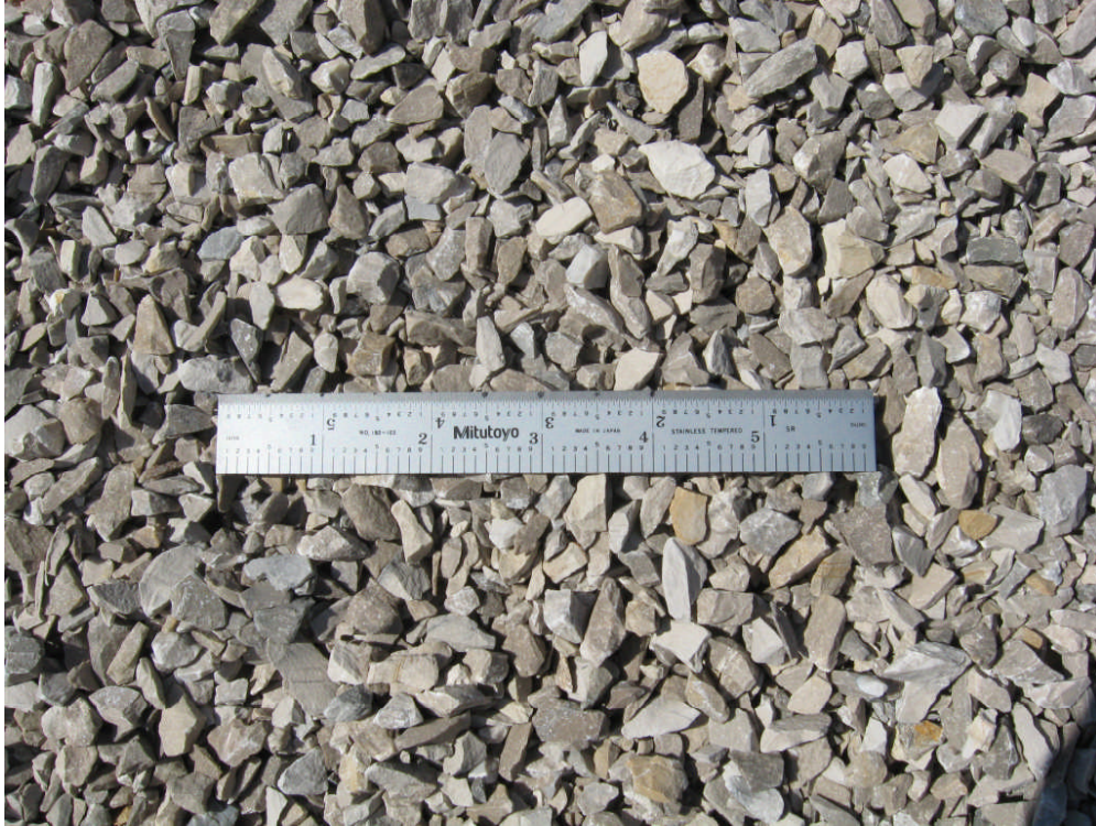
Figure 4-3. Installation damage Type 2 test aggregate.
