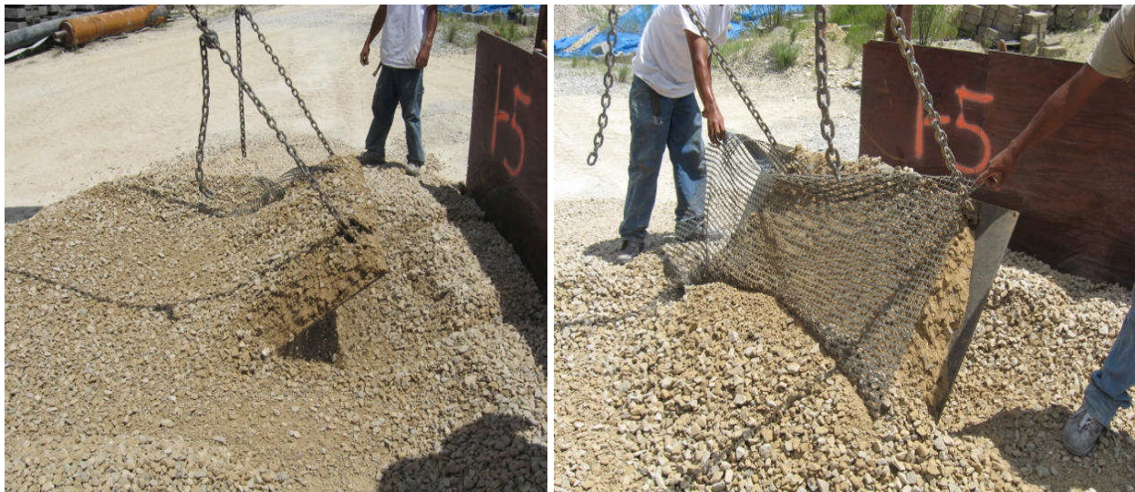
Figure D-10. The steel plates are tilted to facilitate exhumation.
