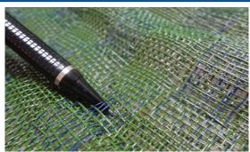
Industry exclusive Pantented Technology creates random pockets within the HPTRM structure to encapsulate and entangle the grass root system.
