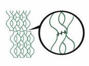
To create a strong seam, apply one staple per inch starting from top or bottom. We offer a hand-held stapler with an extra wide jaw. Use heavy duty staples. Alternately, a pneumatic stapler could be used. For small jobs, drill holes and use 1/4" zip ties instead of staples.
