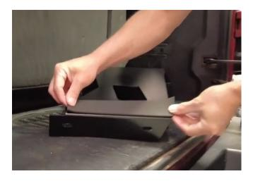
Take 2 of the large bolts and washers and set the driver side wall in place and tighten the bolts to 80%
