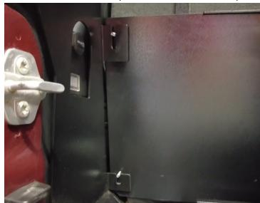
Use 4 spin knobs and put them on the exposed pem studs and tighten them to finger tight.
