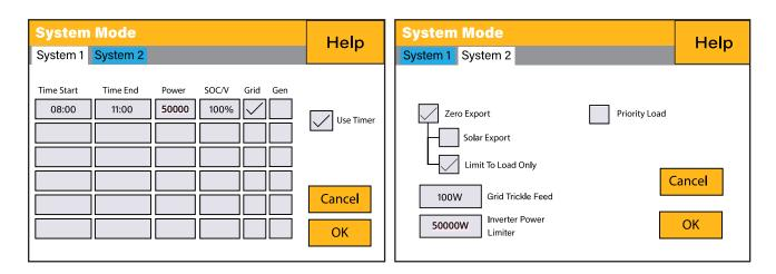
**IMPORTANT** - When charging the batteries from the Grid or Generator, please ensure you have set the correct battery-charging settings on the battery charge as shown in Section 4.10 'Battery Setup' Home Page. If the 'Use Timer' function is activated then the inverter will use the battery power according to your settings when the Grid is present. If this function is not set, the batteries WILL ONLY be used for backup when there is no utility grid power.
