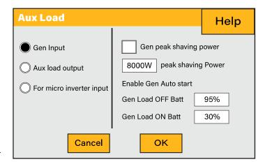
A nice feature of this page is that when the batteries are full and the inverter is still producing power from the solar PV or turbine, it is possible to direct the power generated to another load such as a water heater.
