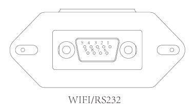
This RS232 port is used to connect the wifi datalogger
