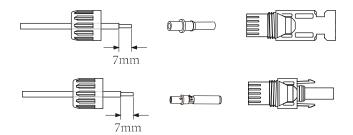
2. Crimp metal terminals with crimping pliers.
