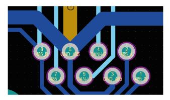
Definition of RJ45 Port Pin for Meter
