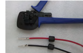
▲ Figure 4.10 Crimp the contact pin to the wire
