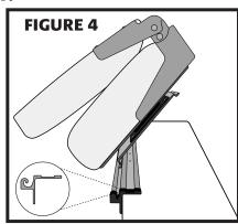
To remove the boat seat for storage, simply lift the back of the boat seat and pull forward until the "C-hook" rotates into its open release position.
