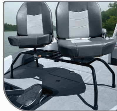
DUAL 3340 QUANTUM SEATS MOUNTED TO 8WD1280 STAND USING KINGPIN HARDWARE
