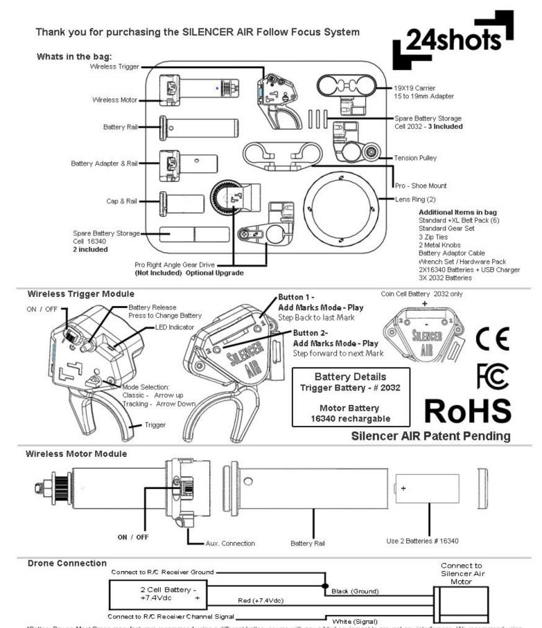
\*Battery Power: Most Drone manufacturers recommend using a different battery source with any added equipment to prevent any interference. We recommend using 2Cell battery pack for the Silencer AIR. Power input 8.5 volts DC MAX. Input wire is ready to be connectorized to your battery. Suggested connection schematic above. We hold NO responsibility for incorrect wiring causing damage to drone, Silencer AIR or any other onboard equipment.
