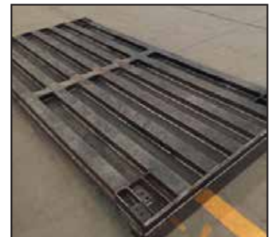
Continuous welding Multiple steel channels
