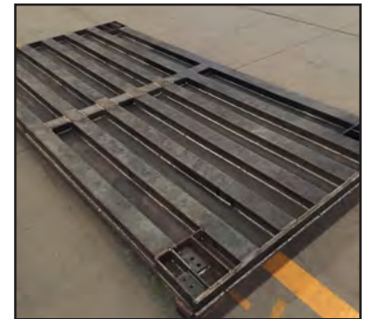
Continuous welding Multiple steel channels
