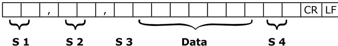
S1: weight status, ST=standstill, US=not standstill, OL=overload
