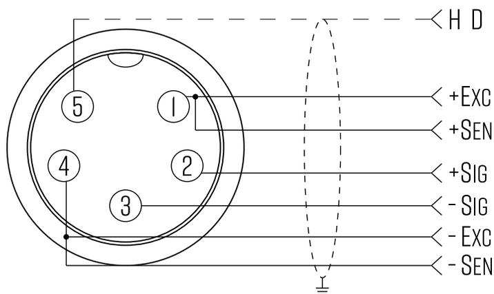
The number of weighing pads and load cells corresponds to the weighing modes. If the pads or load cells are not connected properly the indicator will not function properly. Please use the following table to connect your pads correctly.
