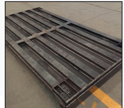
Continuous welding Multiple steel channels
