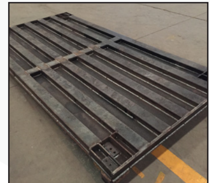
Continuous welding Multiple steel channels
