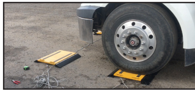
Drive 1st axle over pads
