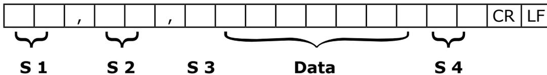
S1: weight status, ST=standstill, US=not standstill, OL=overload
