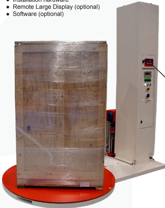
Easy to use OP-900 indicator with 0.9" LED display
