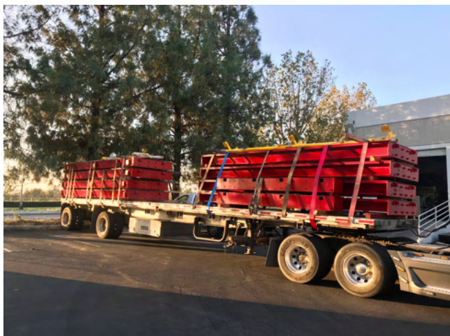
Truck scale panels tied down & ready for delivery
