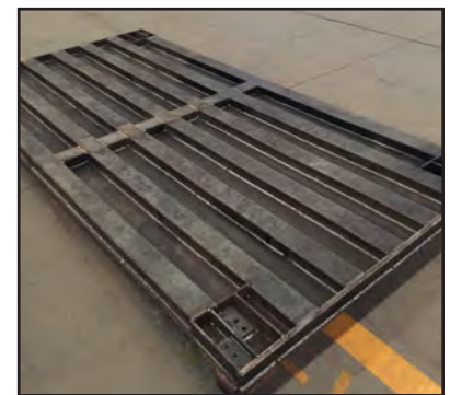
Continuous welding Multiple steel channels
