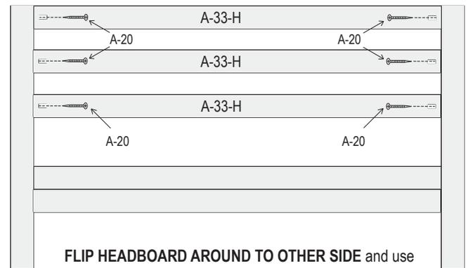
**FLIP HEADBOARD AROUND TO OTHER SIDE** and use screwdriver to secure the (3) A-33-H headboard connectors with (6) A-20 wood screws as pictured.
