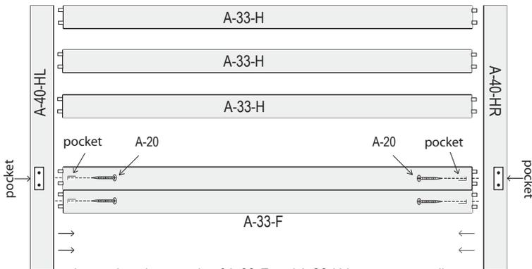
Insert dowels on ends of A-33-F and A-33-H into corresponding holes in headboard legs A-40-HL and A-40-HR as pictured. Be sure pockets on legs and A-33-F bed end are on the same side.
