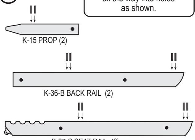
Push Wood Dowels (H-11) all the way into holes as shown.
