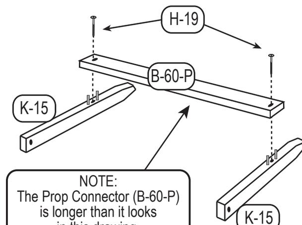
Press the Prop Connector (B-60-P) onto the Wood Dowels on the Props (K-15) and attach with (2) 1-3/4" Screws (H-19).
