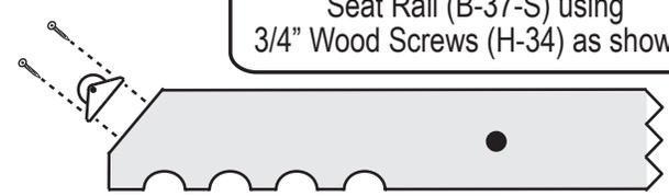
Attach a Wheel (H-LW) to each Seat Rail (B-37-S) using 3/4" Wood Screws (H-34) as shown.
