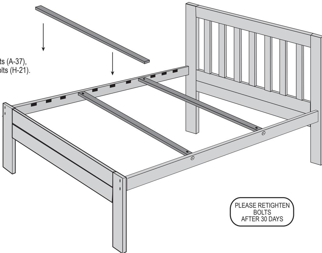
Next insert all Regular Slats (A-37), then tighten the 2 - 1/2" Bolts (H-21).
