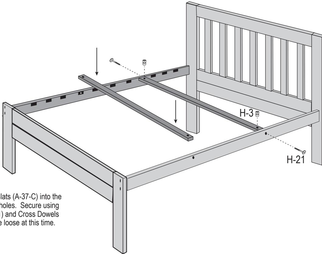
Insert Connector Slats (A-37-C) into the pockets that have holes. Secure using 2 - 1/2" Bolts (H-21) and Cross Dowels (H-3). Leave these loose at this time.
