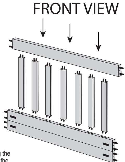
Assemble the headboard by pushing the (7) Headboard Pickets into holes on the Headboard Bottom (A-33-HB) . Then push the Headboard Top (A-33-HT) down onto the pickets
