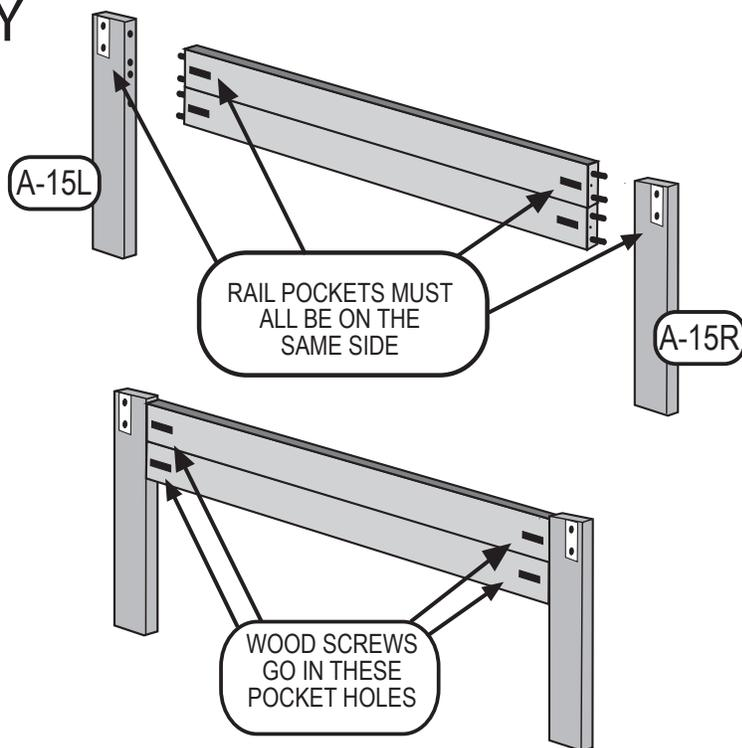
Use a phillips screw driver to attach the Legs to the Bed End using (4) 1 - 1/2" Wood Screws (Black) (H-20).
