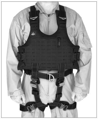
The Helicopter Aquatic Rescue Specialist 2 Harness (HARS 2.0) is a full body water rescue harness with integrated personal flotation. This second generation HARS features design enhancements gained through over a decade of public safety use. The HARS 2.0 features molle compatible panels, stainless steel D-rings, and aluminum side-release buckles for improved durability and function.
