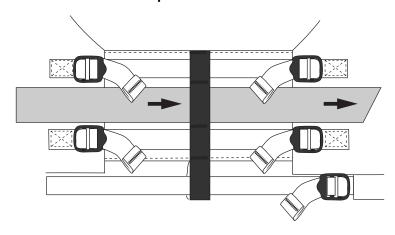
STEP 2 - Thread QR Rescue Belt through web loops and O-ring on back
