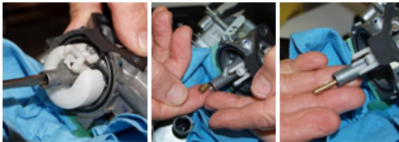
After it breaks lose just unscrew it all the way out. You should have in your hand a small short jet about 3/8" long and a long skinny tube which is the fuel nozzle about an inch long. If the long jet does not fall out tap the metal tube gently to make it fall out and /or squirt some of your carb. cleaner up in the tube to get it to loosen up. This one is not screwed in. Also look and see which end falls out first so you can put it back in the right way. (The end with the bulge faces down.)
