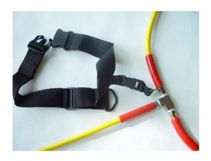
Tow belt attached to the diver hose. (Photo also shows the optional power inflator hose below the tow belt.)
