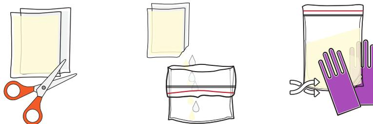
a) Align Resin A & Resin B pouches. Pinch one bottom corner of the pouches to push the resin away and cut an opening.
