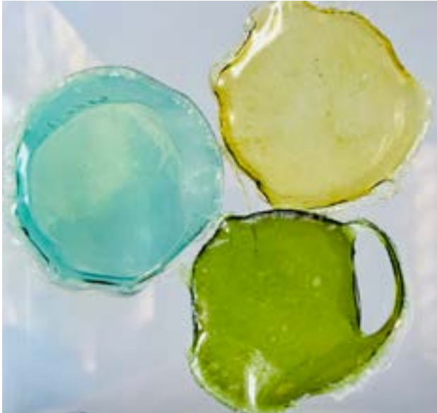
Gelatin-based bioplastics dyed with algae extract.
