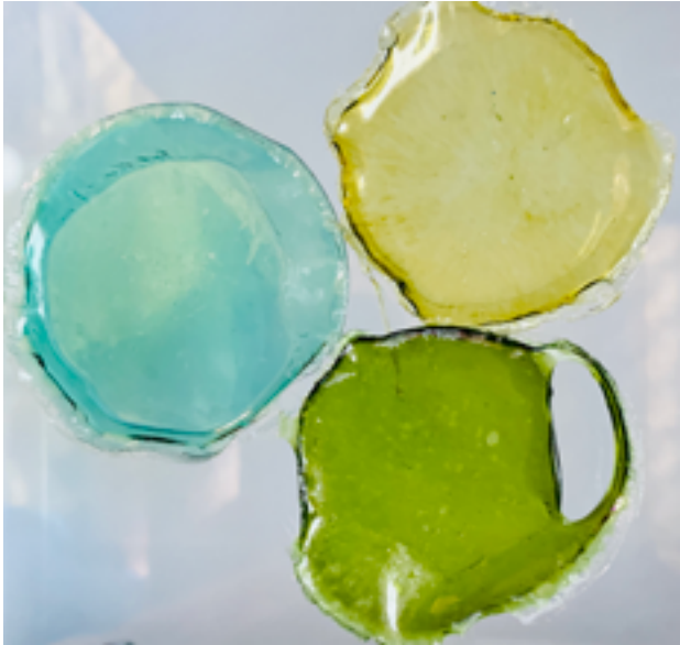
Gelatin-based bioplastics dyed with algae extract.
