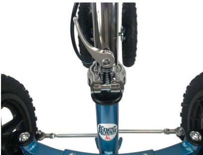
Raise the clamp into the “U” shaped slot
