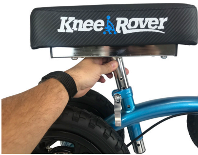
Insert Knee platform into the receptacle tube
