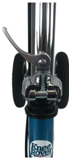
Raise the clamp into the “U” shaped slot
