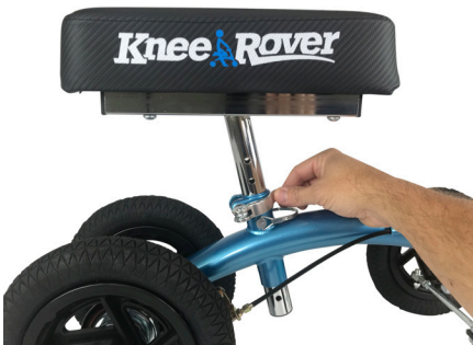
Tighten and secure the clamp
