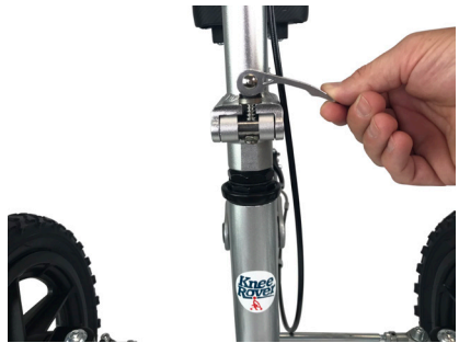
Push clamp down firmly
