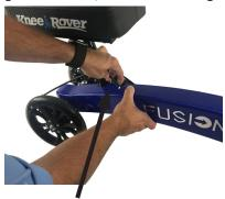
Place brake cable through slot.
