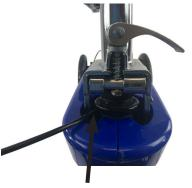
Make sure the brake cable is between the steering column and steering bracket.
