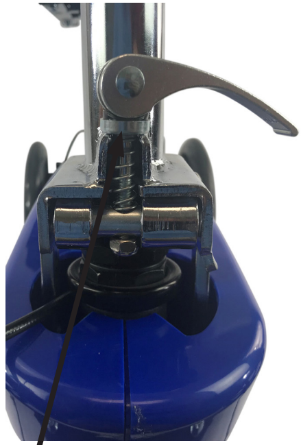
Lever is placed into the “U” slot and clamped down. Steering column is now secure.
