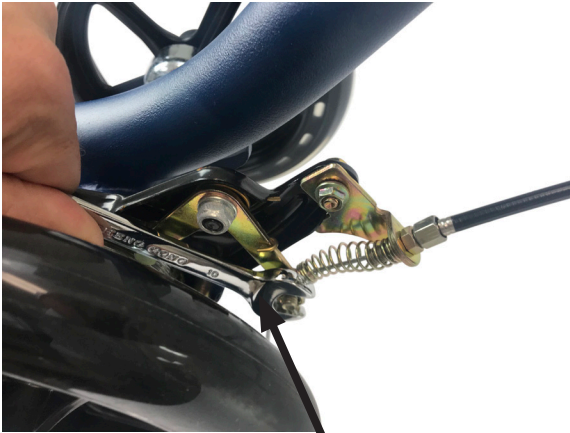
Loosen 10mm nut
