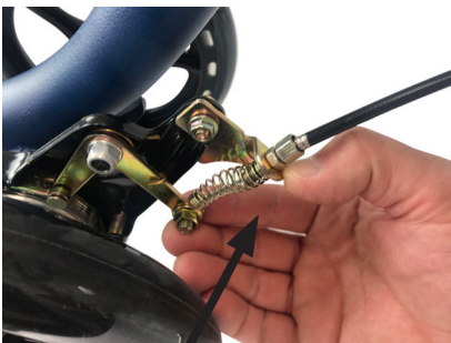
Squeeze spring together and pull the brake cable
