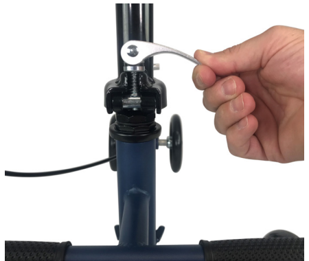
Push clamp down firmly
